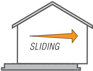
When wind blows against the side of the structure, exerting a lateral force that causes the structure to slide off its foundation.
