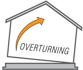
When the structure is anchored in place to limit racking or sliding, the lateral force of the wind causes the structure to rotate or overturn.
