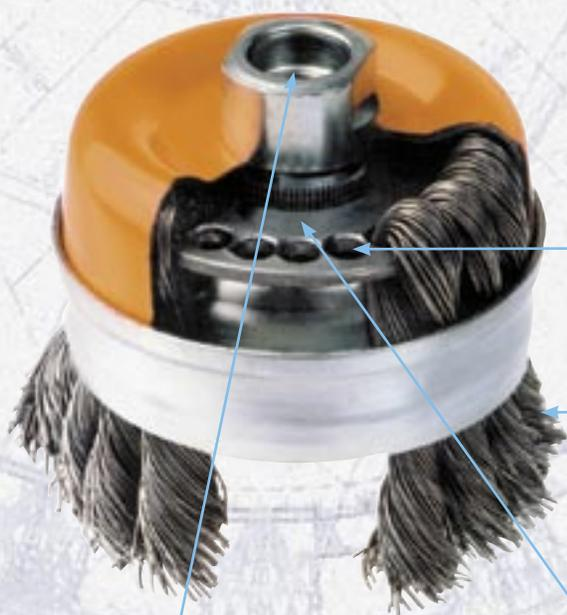
Every knot is perfectly balanced through accurate wire count and even trim length before being permanently anchored in an individual hole. This ensures perfect concentricity and vibration-free brushing for maximum operator comfort.
