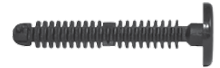
247-240 Std. Pkg. 25 pcs. Head Dia. 11mm, Stem Length: 35mm FORD Radiator Attaching Retainer Fits into 4.75mm Hole, Panel Range: 5-29mm #N-800505-S
