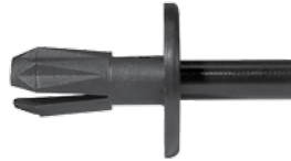
247-460 Std. Pkg. 25 pcs. Head Dia. 3/4", Stem Length: 11/16" FORD Truck 1978-on Grille to Metal Stamping Retainer Shoulder Length: 1/4", Fits into 1/4" Slot #387944-S CL Part No: 910-0795, Pieces: 2
