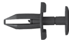
247-417 Std. Pkg. 25 pcs. Head Dia. 17mm, Stem Length: 16mm GM C&K Truck 1999-on Fender/Front Bumper Cover Retainer Fits into 6mm Hole #15149708 CL Part No: 910-0605, Pieces: 2
