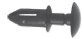
247-412 Std. Pkg. 25 pcs. Large Head Dia. 3/8", Stem Length: 7/16" GM Tail Light Retainer Fits into 3/16" Hole #16500308
