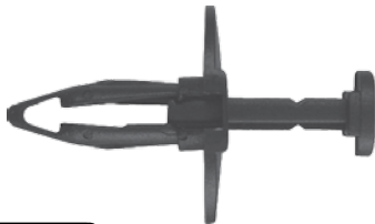
247-467 Std. Pkg. 25 pcs. Head Dia. 1", Stem Length: 7/8" FORD Fascia Retainer Shoulder Length: 1/8", Fits into 5/16" Hole #N803421-S CL Part No: 910-0635, Pieces: 3
