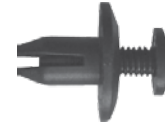
247-491 Std. Pkg. 25 pcs. Head Dia. 15mm, Stem Length: 11mm HONDA Push Type Retainer Fits into 6mm Hole #90684-SA5-0030
