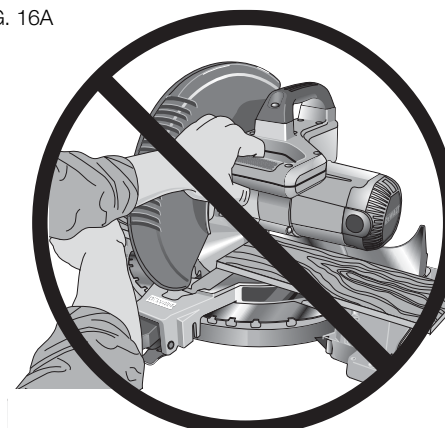
IMPROPER HAND POSITION
